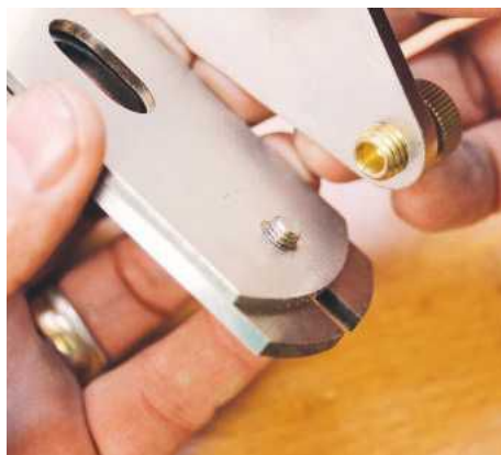
▲ A longer screw on the iron acts as a stud to connect to the lever cap screw
